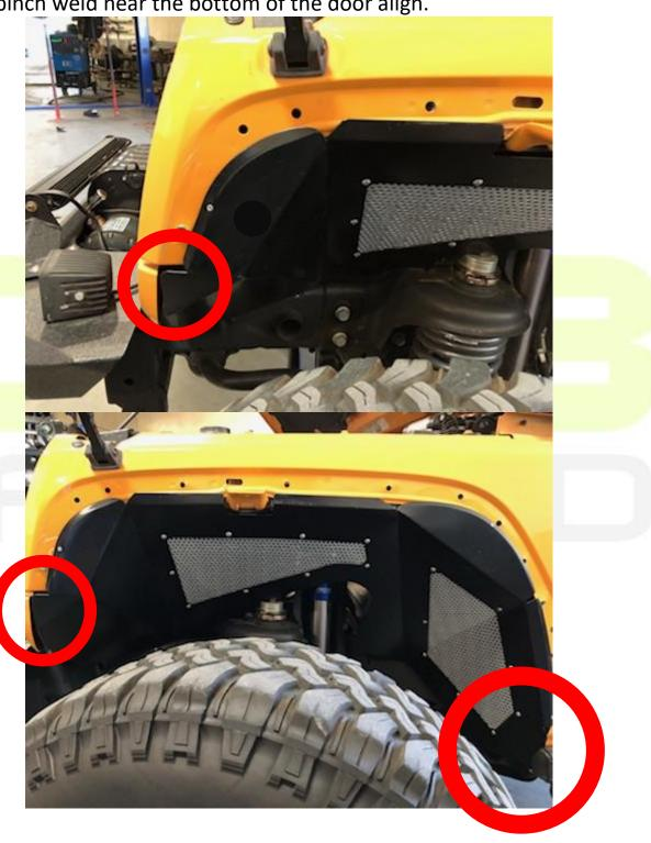
**6.** Once aligned, mark holes in inner fender on Jeep body. Using 1/8" drill bit, drill marked holes in body. The inner fender will sit on top of the edge of the wheel well.
