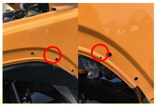
7. Realign inner fender. Using rivet gun and provided rivets, install the inner fender. Ensure proper inner fender alignment prior to install rivets.
